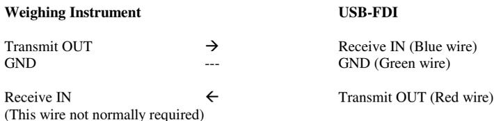
Typically the weighing equipment should be set up to send out a serial string at the desired baud rate and parity each time the PRINT key is pressed.
